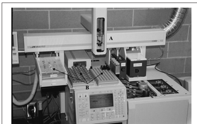
Figure 9. Commercial SPME–GC autosampler (CTC Analytics CombiPAL): sample preparation/injection arm (A), sample trays (B), needle heater (C), and heater/agitator (D).
